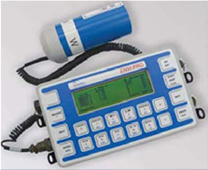
Figure 7: Scintrex Envi Pro proton precession magnetometer.
